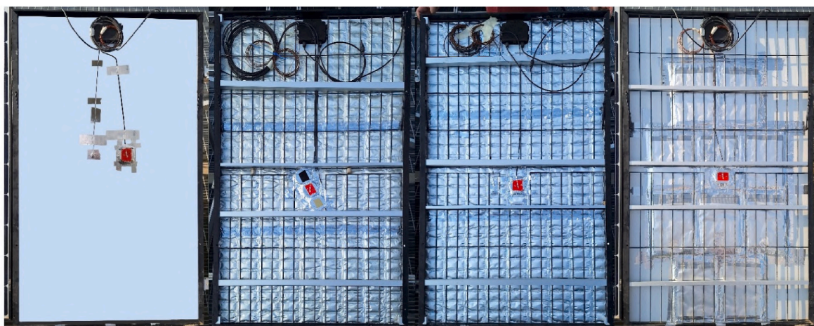
Fig. 2. Back surface view of the reference PV and PV-PCM modules.
